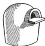
FIG. 2.—Covered pot for glass melting, as used for flint glass and optical glass.
