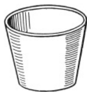
FIG. 1.—Open "pot" or crucible for glass melting.
