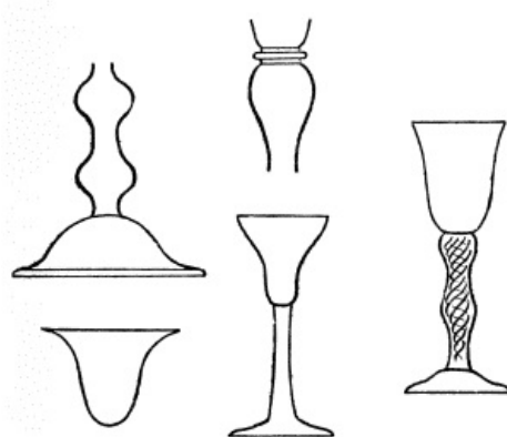
FIG. 42. The figures given above illustrate certain of the characteristic features of Old English glasses. Thus Fig. 1 is an example of a double-knopped stem, each of the bulges being technically known as a "knop." The foot is "domed." No. 2 is an illustration of a shoulder and collar, the shoulder being the bulge near the top, and the collar the ring above it, which was originally devised to hide any clumsiness in joining the stem to the bowl. No. 3 is a "flanged" bowl, No. 4 a "waisted" bowl, and No. 5 shows an air-twisted stem.
