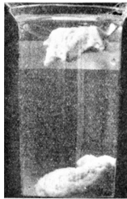
Gluten in water containing both acid and sulphates. It shows varying degrees of coherence, but is brittle or "short"
