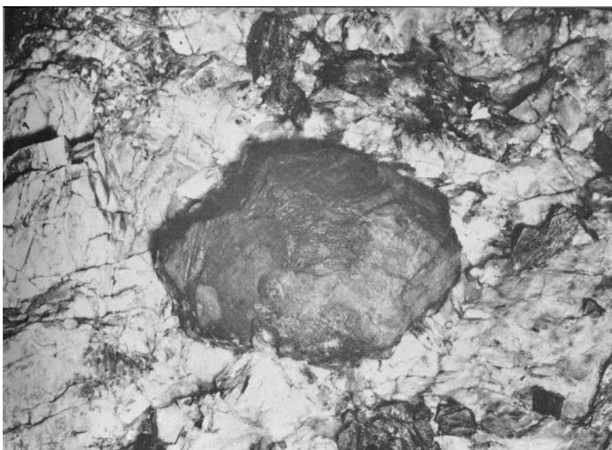
Figure 25. Garnet crystal in pegmatite. The crystal is about 6 inches in diameter. Other minerals are feldspar (white) and clusters of white mica flakes. The mica crystals appear dark in the photograph because they
