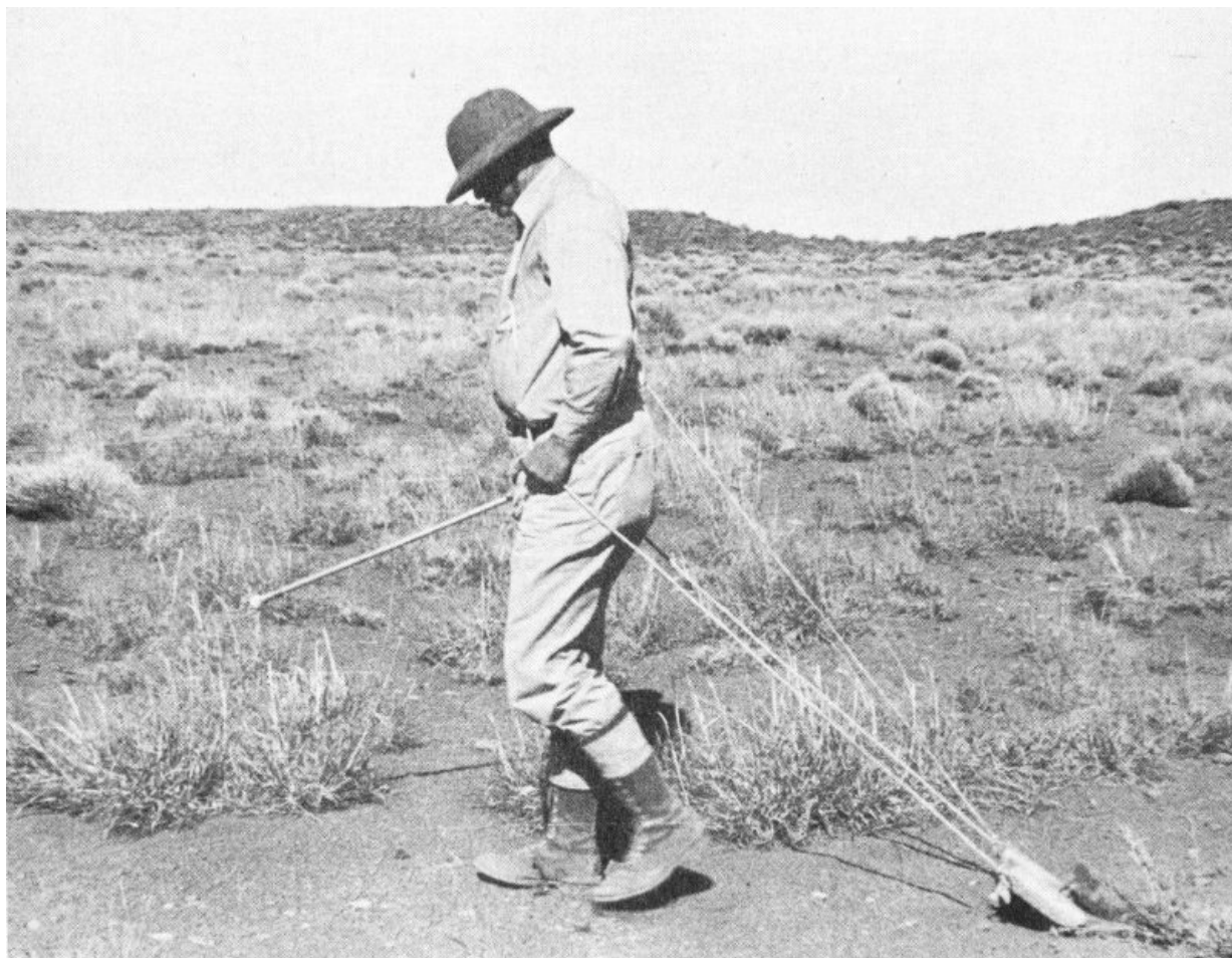
Collecting small surface specimens of meteorites with portable detecting devices: a powerful alnico magnet mounted on a light wooden sled, and a horseshoe magnet at the end of a cane. See p. 98 . 97
