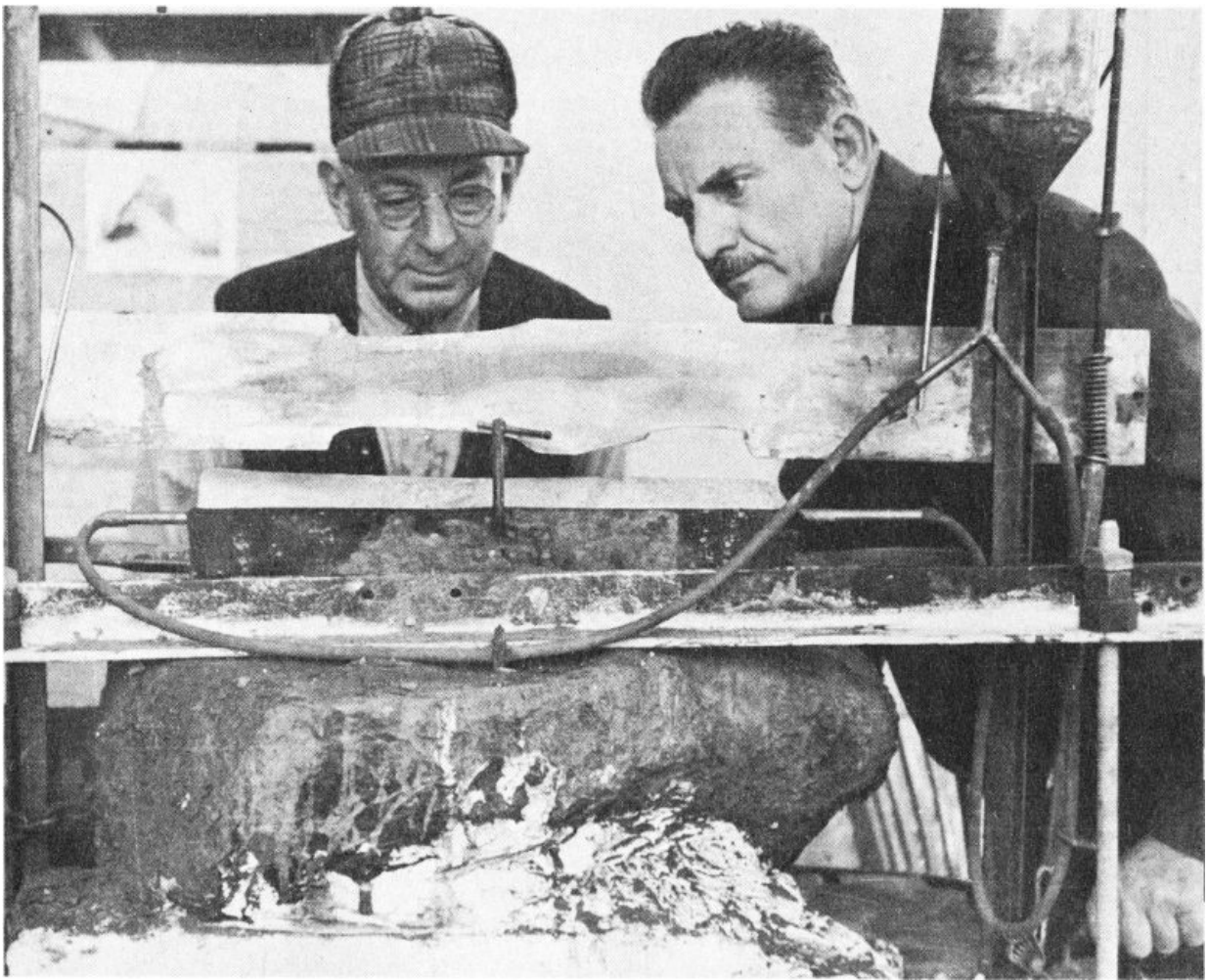
The Lake Murray core mounted on the meteorite saw which cut it in half. One of the worn soft iron saw-blades is held above the meteorite by the saw guides. See pp. 167 , 168 .
