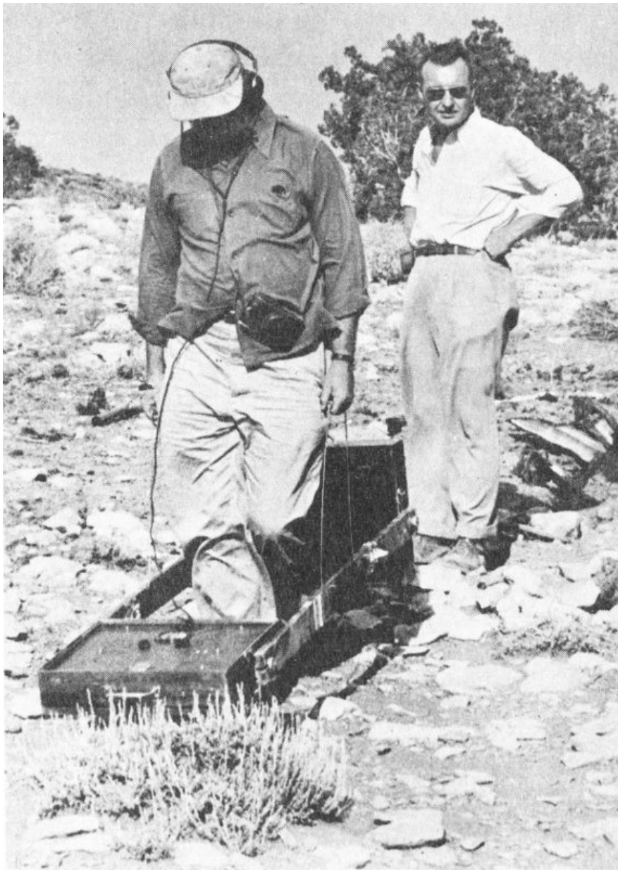
A commercially built meteorite detector in operation.
