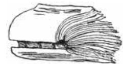
FIG. 39.—What a book may do if the back is not properly rounded.
