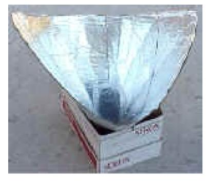
[Image: 01.jpg -- Photo description this image shows a cardboard box being used to support a silvery funnel, roughly 3 feet high. The funnel is placed within the box so that the sides of the box hold the funnel upright. Sitting within the base of the funnel is a black jar inside a clear plastic bag. The plastic bag is inflated like a balloon to seal an insulating air pocket around the jar.]
