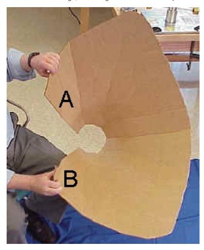
[Image: 05.jpg -- Photo description: This is looking strait down into the mouth of a cardboard funnel. A man grabbed what was the long edge of the sheet of cardboard, now divided in two by the half circle cut from it. The two now separate edges are now brought together to form a cone. The cone has no tip because of the cut-out half-circle.]
