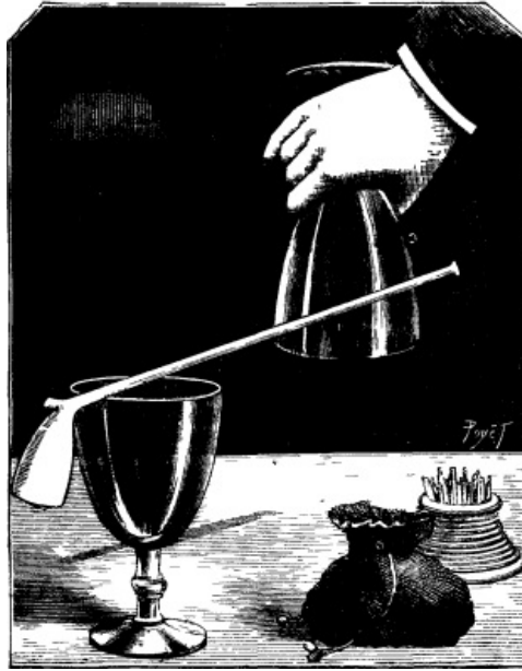
CLAY PIPE ATTRACTED BY AN ELECTRIFIED GOBLET.
